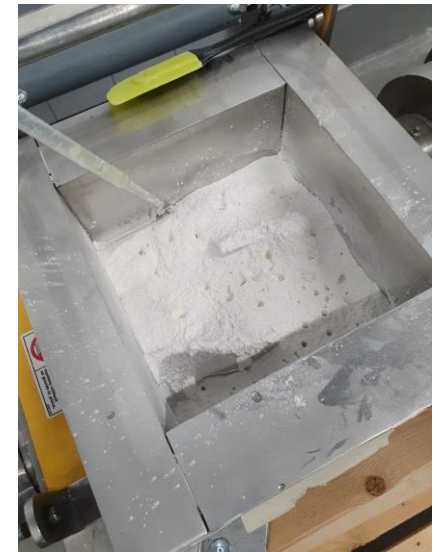
Mixing of oil with CNF powder in z-blade mixer
