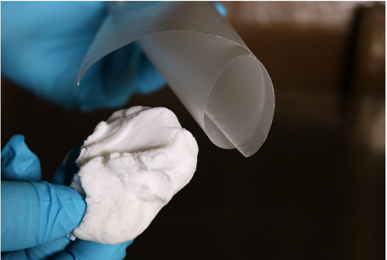
Description: A ball made from nanocellulose from which the biomaterial film was produced. Source: copyright VTT
