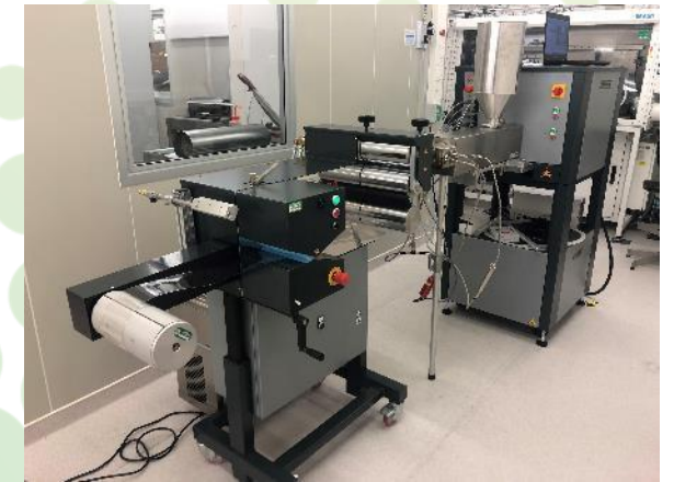
Single screw extruder equipped with a flat die and a calendaring system
